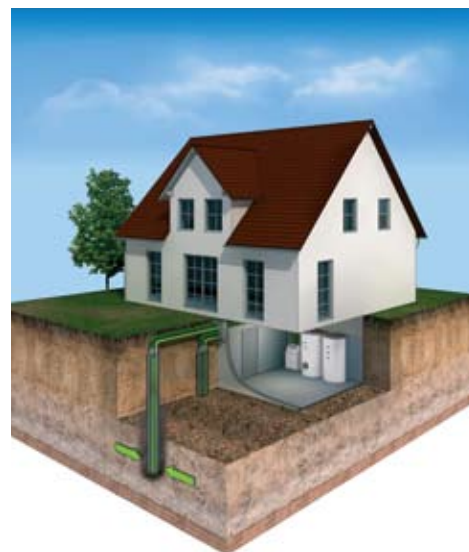
Ground/water system (vertical geothermal probes)
