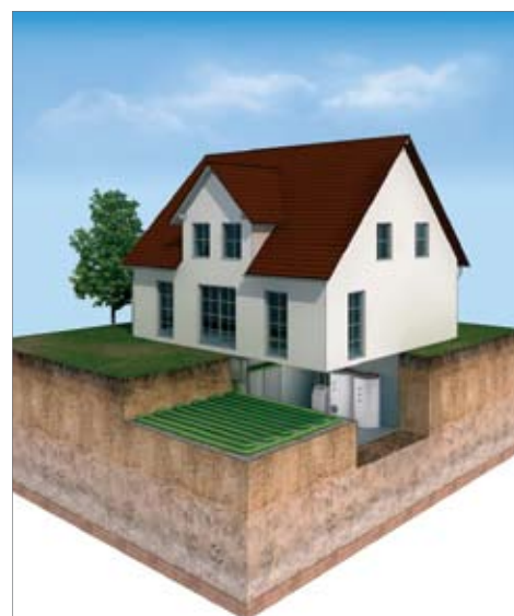
Ground/water system (horizontal ground collector)
